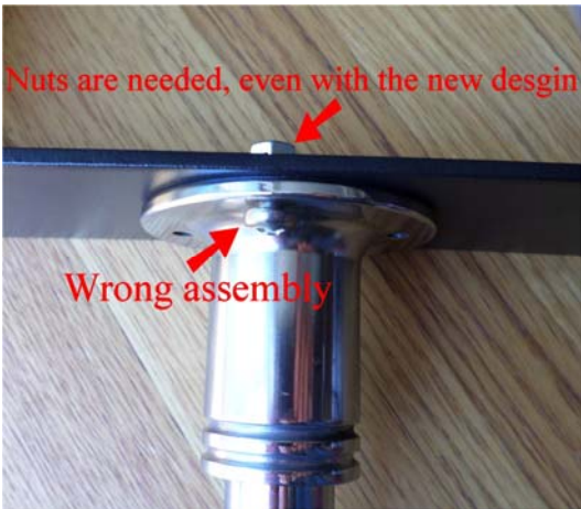
Figure 10. The wrong way
