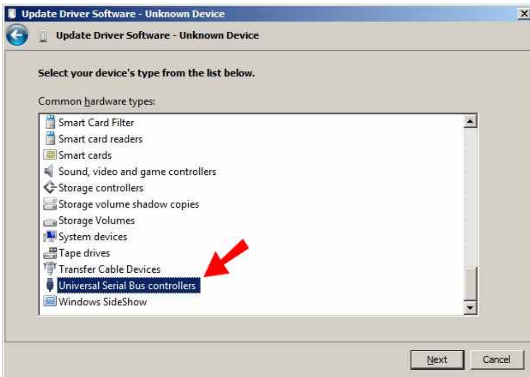
Figure 3. When this screen comes out, click “Universal Serial Bus Controller” pointed by the red arrow and then click “Next”.
