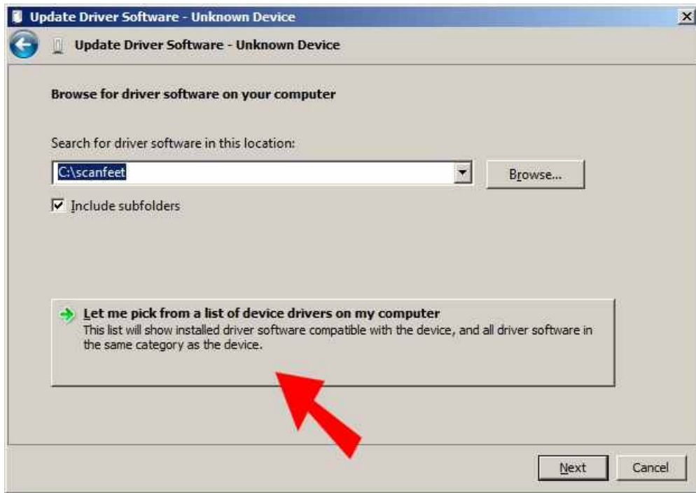
Figure 2. When this screen comes out, click “Let me pick from a list of device drivers on my computer” pointed by the red arrow. This is different than our usual method, which asks the user to click the “Browse” button to search for driver and the “driver cannot be found” message comes out.
